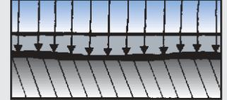
*Electrical attraction causes negatively charged paint particles to be attracted to positively charged structural steel, forming a smooth even finish.*
